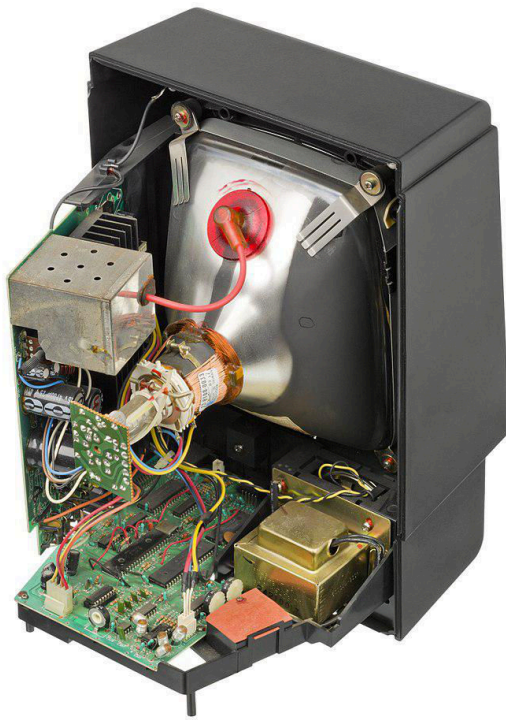
Fig. 4 - Interior view of the Vectrex: the side board contains the power management while the bottom board is the console motherboard (author: jesmar - source: Festival du Jeu Video)
